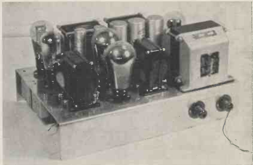
HOW THE AMPLIFIER SECTION IS ARRANGED The amplifier unit contains the whole of the low-frequency portion of the set, together with the mains-rectification and smoothing circuits. The plugs and sockets are for the mains input and a spare one for use if required
