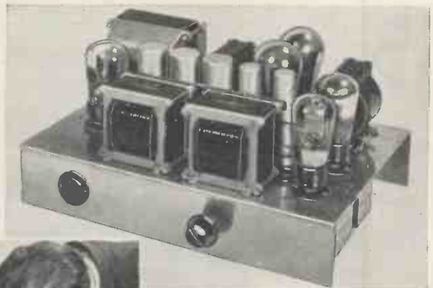
FRONT VIEW OF THE AMPLIFIER The control on the right is the tone compensator and the valve-holder socket is for inserting the plug which carries high- and low-tension current to the radio unit
