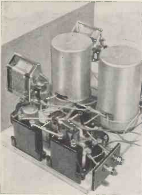
LOW-FREQUENCY SIDE This close-up photograph shows the low-frequency side of the set. It will be noticed that the fixed resistances are suspended in the wiring
