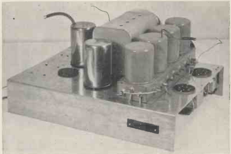
ANOTHER BACK VIEW OF THE RADIO UNIT This photograph emphasises the simplicity of the radio unit. The set has been designed so that the beginner with little experience at set construction will find building a really easy job. The metal chas. is can be obtained ready drilled
