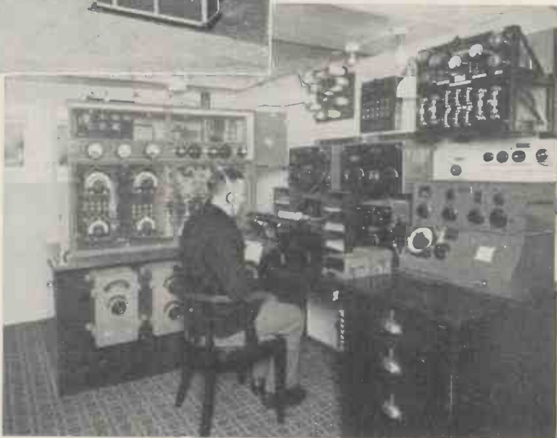
Here is a corner of the radio room on board the C.P.R. liner, "Empress of Britain." On the left is the long-wave telegraphy transmitter, and on the right is the latest Marconi direction-finder, a fine aid to navigation
