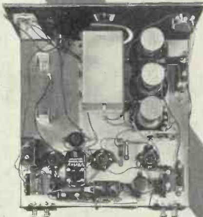
A plan view of the set showing the disposition of the parts. The coils and three-gang condenser are supplied as a complete assembly on a metal baseplate
