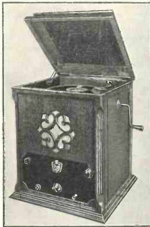
CONTROLS OF THE HARRIS ETHERGRAM The two knobs in the top left-hand and right-hand corners are for controlling volume and reaction respectively. Along the bottom of the panel are the wave-change switch, the main tuning knob, and the on-off switch. The gramo-radio switch and the tone control are mounted on the motorboard, the gramophone volume control forming part of the pick-up
