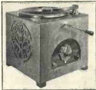
A TWO-VALVE RADIOGRAM The New Style Radiogram described in the October issue of "W.M." is cheap to build and gives fine results
