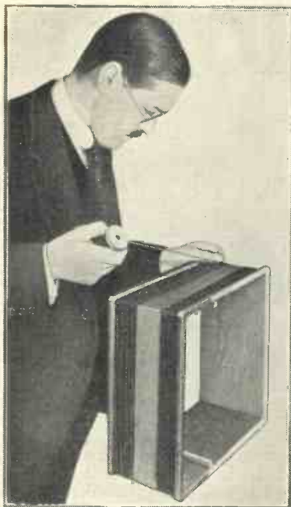
WINDING THE FRAME AERIAL
