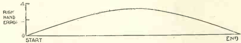
Fig. 7.—Compare this with Fig. 6: it is to the same scale, and shows the error for a 10-in. tonearm arranged as in Fig. 5
