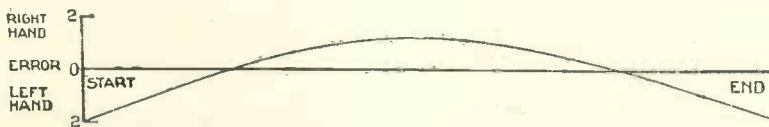
Fig. 8.—By slightly altering the offset angle the error is reduced still further—to 2 degrees for a 10-in. tonearm
