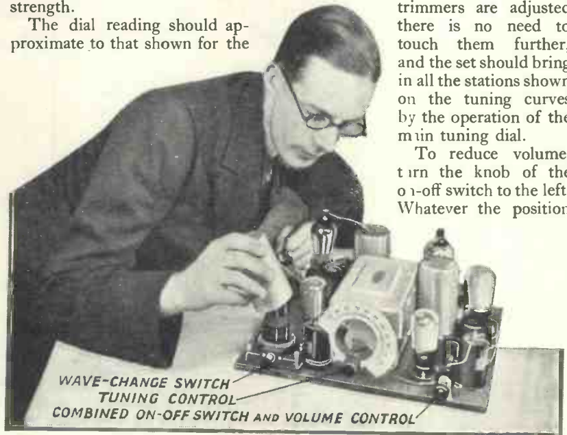
ONLY ONE KNOB TO TUNE—THREE CONTROLS IN ALL
