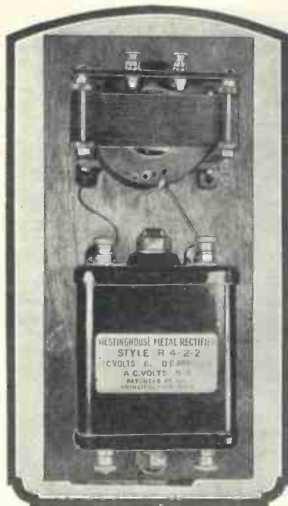
Plan view of the one-ampere charging unit. The dry rectifier is a Westinghouse type R4-2-2. Transformers already built up can be obtained from the Regent Radio Supply Co., or, if desired, the reader can obtain Stalloy stampings and a bobbin for winding his own transformer from the same firm
