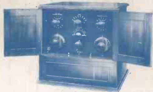
4-VALVE SET. —300-4000 metres Duostat control for Dull Emitter or Bright Emitter Valves—1 H.F. with tuned anode—1 Detector, 2 L.F.—Retroactive tuner with the most efficient reception over the whole range of wavelengths. The last valve is suitable for power amplification.
