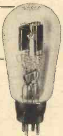
The Osram U.10, a general purpose full-wave rectifier.
