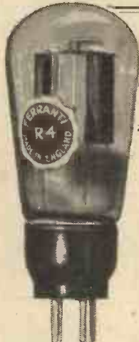
This Ferranti full-wave rectifier gives an output of 120 m.a. at 250 volts.
