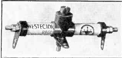
A miniature version of the popular Westinghouse metal rectifier, the "Westector," makes an excellent second detector for superhets. The model above is for full-wave rectification.
