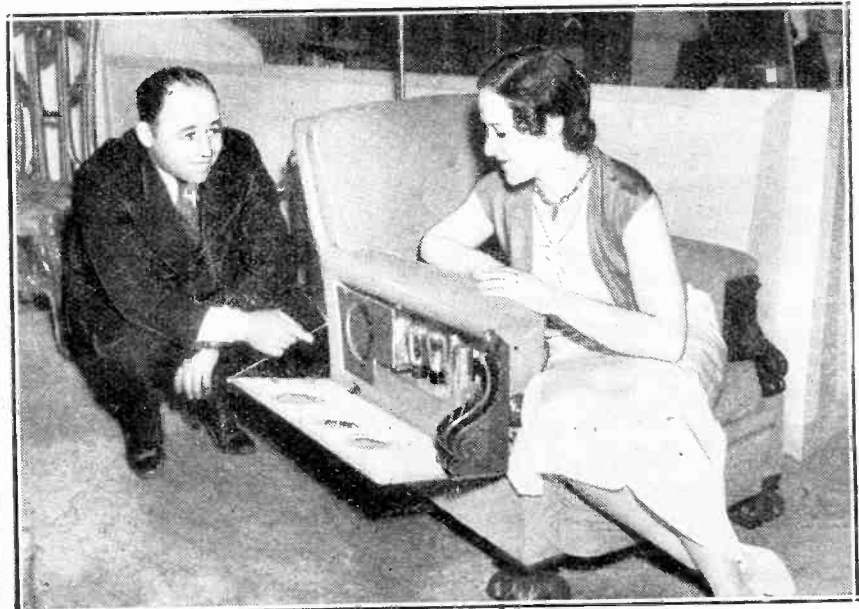
It is entirely contained in the arm of the chair, so it can be tuned and adjusted whilst lying back at full ease.
