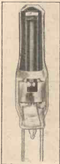
To the left is a Marconiphone "Catkin," part of which has been cut away to show the internal construction. The valve on the right is a non-metallised M.H.4, the characteristics of which for various anode voltages, etc., are shown in the central graph.
