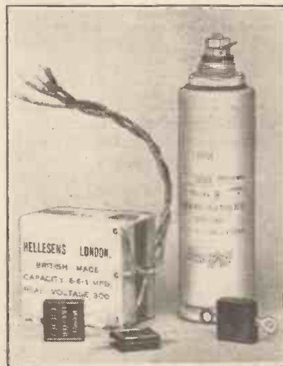
In the above photograph are shown samples from the extensive range of Hellesen condensers. The "pack" is of the dry electrolytic type, and on the right is an 8-mfd. wet electrolytic condenser designed to withstand a 500-volt peak. The three small fixed condensers in the foreground have ruby mica dielectrics.
