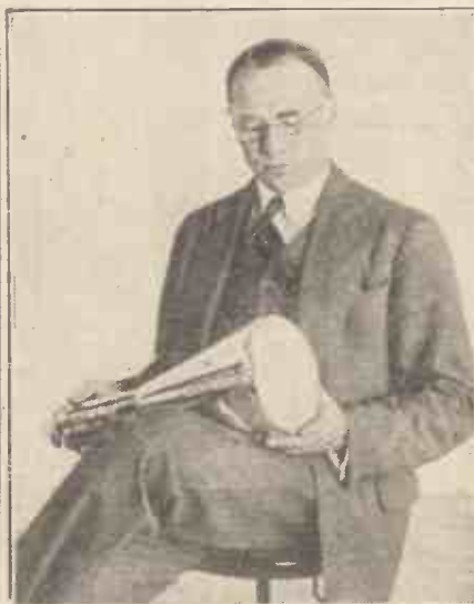
The use of the cathode-ray is one of the latest methods of attacking the television problem, the picture appearing at the round end of a cathode-ray tube. Such tubes are similar to the one shown in the above photograph.
