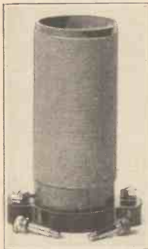
The new Ward & Goldstone type W.H.F. heavy duty choke designed for use in D.C. mains circuits. Having a D.C. resistance of only .75 ohm, the winding is still capable of carrying up to .6 ampere.
