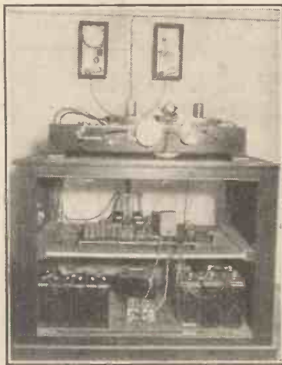
This is the ingenious device which answers telephone calls in Paris and automatically speaks the hour and minutes to the subscriber who inquires.
