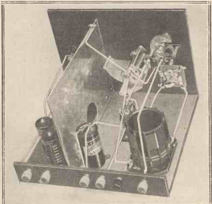
The coil in the set with which the adaptor is employed operates in place of the second "S.T.300" coil, for Mr. Scott-Taggart always aims at reducing costs.
