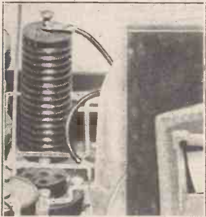
The practice of using a flexible resistance to act as a connecting lead (as well as provide the necessary ohms) sometimes results in the temptation to stretch it a little, or to bend it round other components out of the way. This is bad practice, and the Spaghetti should always be arranged loosely, as shown here, with no strain on its tags.
