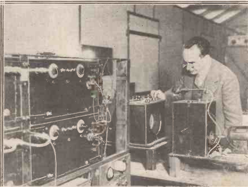
This apparatus at Slough is used for keeping a record of lightning flashes, and has a range of many thousands of miles. It is really a very powerful radio receiver, designed specially for the reception of atmospherics.
