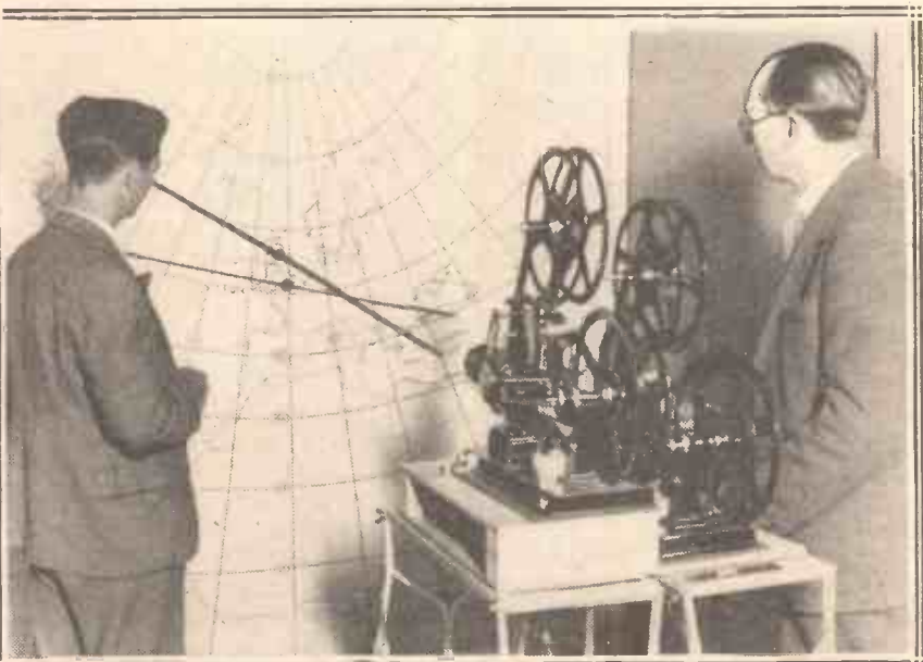
This film projector is used to locate lightning flashes recorded on cathode ray direction-finders, employed by the Radio Research Board. It keeps watch on the thunderstorms of a whole continent.
