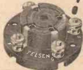
TELSEN VALVE HOLDERS , Pro. Pat. No. 20286/30. An entirely new design in Valve Holders, embodying patent metal spring contacts, which are designed to provide the most efficient contact with the valve legs, whether split or NON-SPLIT. Low-capacity, self-heating, supplied with patent soldering lugs, and hexagon terminal nuts. Fitted with nickel-silver shock-absorbing spring contacts. Price 1/- each.
