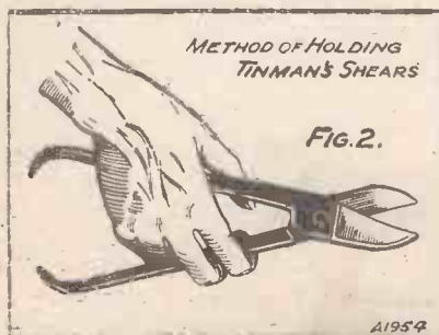
This is how Mr. Hallows advises you to manipulate the cutters.
