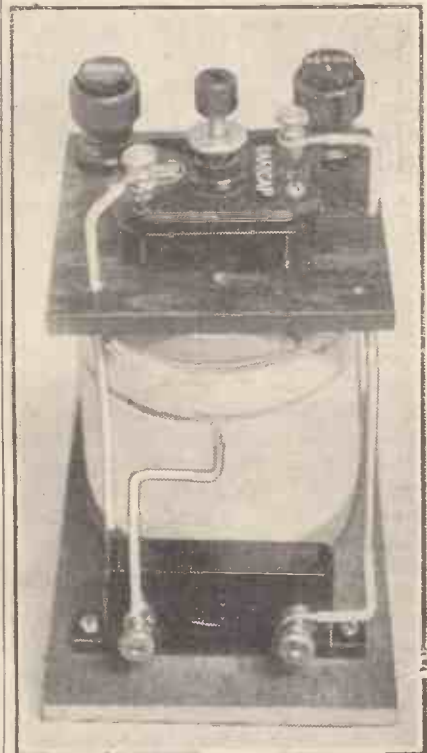
There is only the one little adjustment. You turn that little condenser knob until your interfering station is suppressed.
