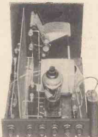
This is a photograph of the "S.S." H.F. unit, which can be added to any set. It was described in last month's "Wireless Constructor." Note the grid bias!
