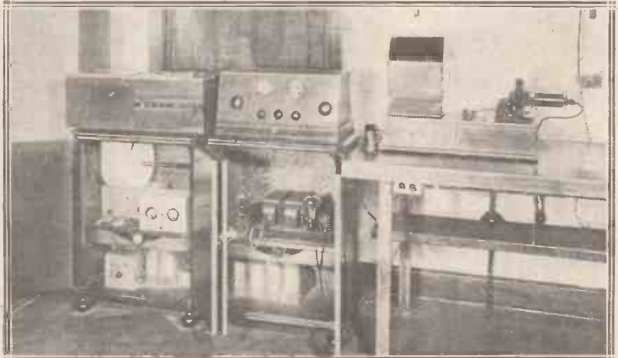
A general view of an automatic response-curve device which provides a means of "looking" at the reproduction of a loud speaker. (Ultra Electric, Ltd.)
