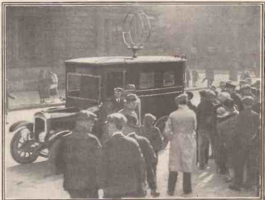
The Post Office wireless detector van leaving Glasgow on a tour of Scotland to search for radio oscillators.
