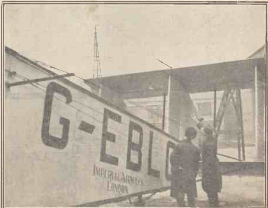
So that the airman need not wind in his aerial when nearing the ground, on each new Imperial Airways' machine a 3-wire permanent aerial is stretched between the wings and tail, as shown in this illustration.
