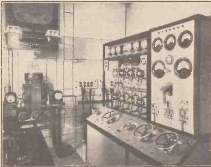
The main control panel of the Marconi transmitter employed at the Lausanne broadcasting station. It operates on 680 metres from 8 p.m. onwards.
