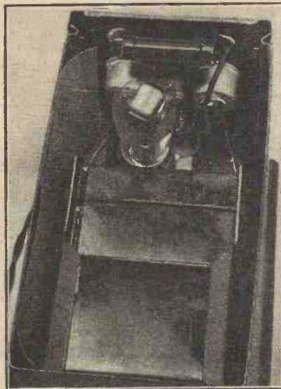
Interior of the Majestic Unit showing the voltage control, resistances and rectifying valve.
