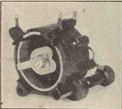
The method of mounting the filament resistance on the Harlie valve holder.
