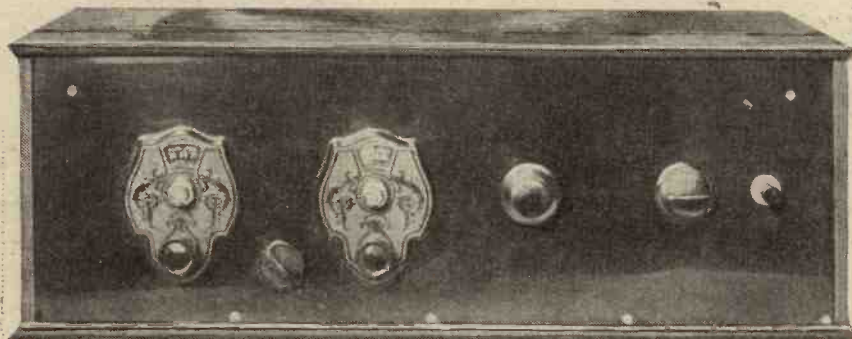
Next to the main tuning dials are the reaction and volume controls. The on-off switch is on the extreme right.
