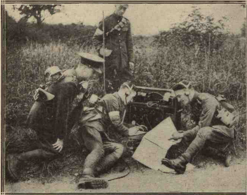
Radio and the Army. One of the wireless sets used to link up field guns with the front line.
