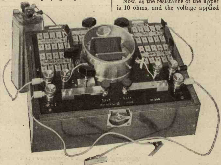
The Wheatstone Bridge employed for the measurements described in this article
