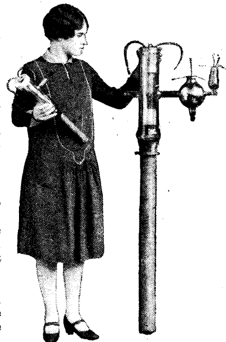
Compare the 20-kw. valve in the girl's hand with the latest 100-kw. type used at W.G.Y.
