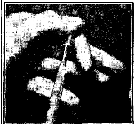
The screwdriver should be kept straight, and its blade edge snugly pressed into the slot of the screw.
