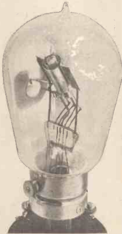
An example of modern design: the K.L.1 valve, designed to operate off A.C. mains.
