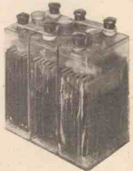
The white marks on this accumulator show where the plates have "sulphated" owing to neglect.
