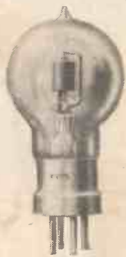
An old type of bright emitter "R" Valve, which used to be employed in all stages of receivers a few years ago.
