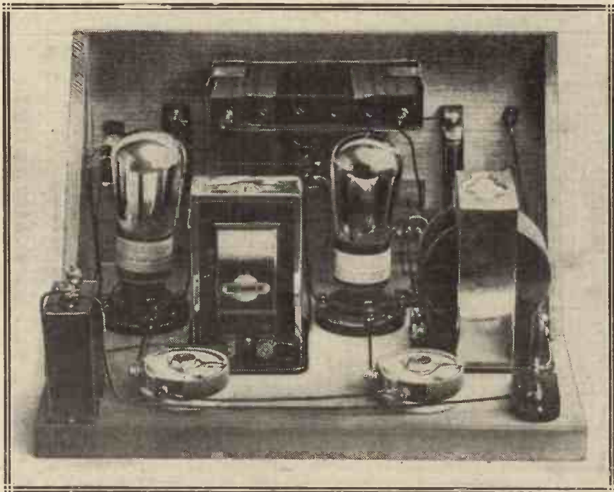
The complete amplifier with grid bias battery and valves in position, ready for housing in its cabinet.
