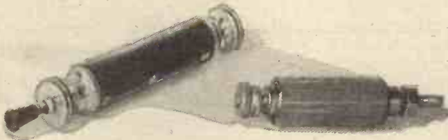
Two examples of permanent detectors, the one on the left being capable of adjustment should this be deemed necessary.
