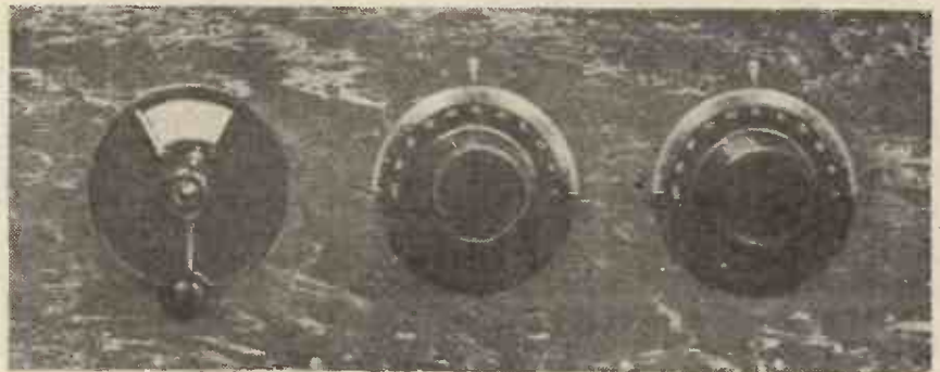
The three condenser controls and two terminals are the only components which appear on the panel of the "Selector Two."
