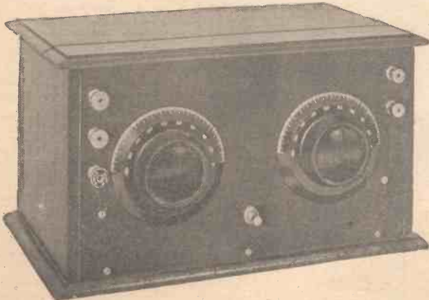
The tuning and reaction-condensers, and an on-off switch, are the main features of the panel, all being readily accessible.
