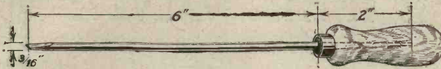
Fig. 3.—A long-handled screwdriver is much more easy to use than one of ordinary type.
