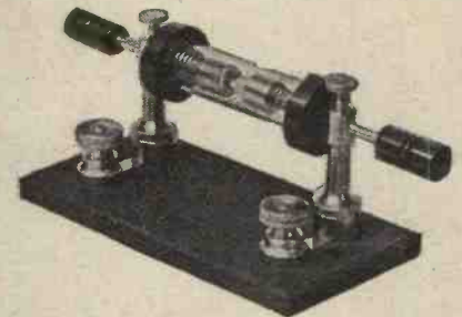
A double-crystal detector in which the positions of both crystals are adjustable.
