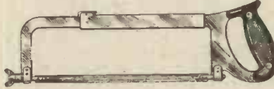
Fig. 2.—A comfortable and steady grip may be obtained with a handle of this type.
