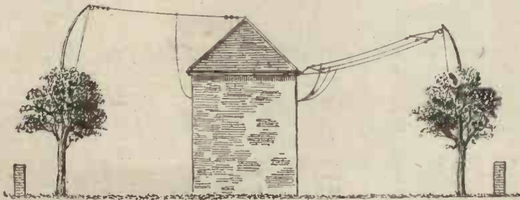
Fig. 1.—Many badly erected masts are ugly, if not dangerous, especially when no stays are employed.
