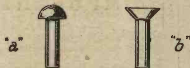
Fig. 3.—Two forms of rivet, namely cup-head and countersunk-head, respectively.
