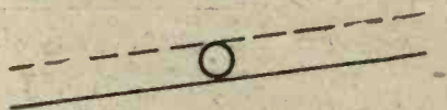
Fig. 2.—The method of synchronisation adopted in the Anstey system depends upon the rolling of identical balls down similarly inclined paths. (See D in Fig. 1.)
