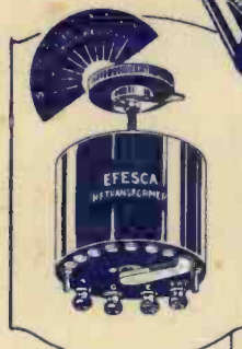
EFESCA TUNED ANODE An alternative method to H.F. Transformer Coupling. Must be used in conjunction with a variable Condenser of .0003 to .0005 mfd. Wavelength range 150 to 2,600 metres. 21/- each.
