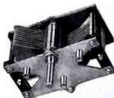
No. 301-A Low Loss Condenser. Grounded rotor type with straight-line curve. Capacity range .000009 to .0005. For use with No. 105 and No. 205 coils. Price $4.50
