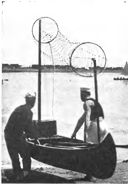
Radio signals transmitted from an antenna of this type spread out in all directions
