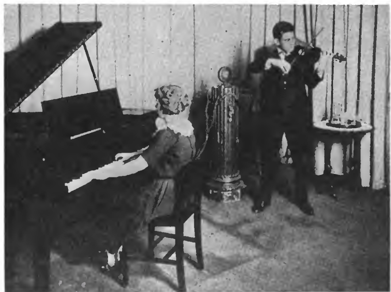
In converting sound into electricity in broadcasting for instance, the music is first picked up by a microphone located near the instruments. In this case the microphone is concealed inside the circular housing which is on top of the pedestal
