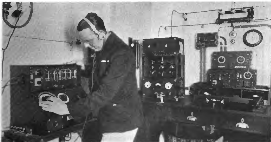
A corner of the operating room on the "Majestic," showing Third Radio Officer Brunt at one of the special receivers, used for direction finding. In the center is the big 1½ kw. continuous wave transmitter, and at the right the ordinary receiving apparatus
