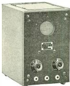
Type DA Tube Detector and Two-Stage Amplifier
