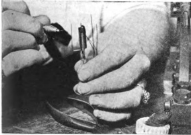
Anchoring the filament to one of the supporting leads by a tiny wire hooked under the end of the filament and welded to a support
