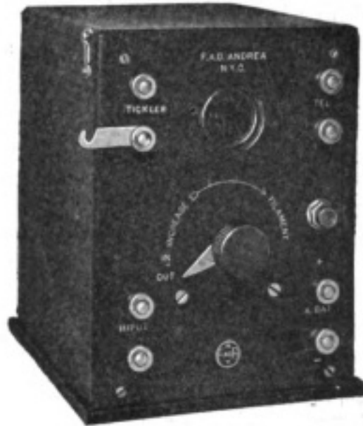
DETECTOR CONTROL PANEL
