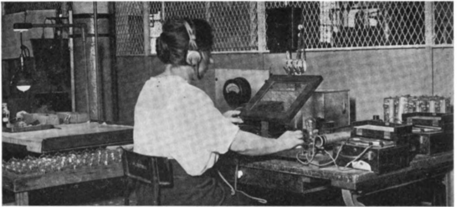
Testing detector tubes under actual operating conditions before shipment
