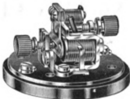
Illustration Shows Buzzer With Metal Cap Off
