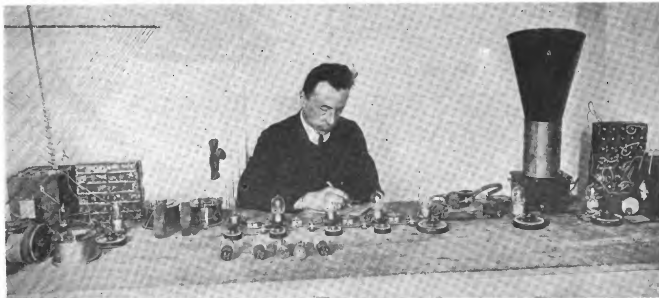
Complete arrangement of apparatus used in the Armstrong short wave amplifier, showing nine VT'S, one used as a detector, one as an oscillator, five as radio-frequency amplifiers and two as audio-frequency amplifiers
