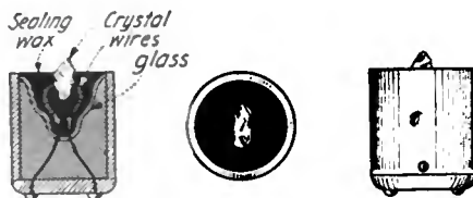
Details of the sealed in detector
