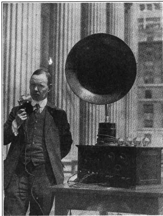
Int'l Film Service The "Magnavox"—meaning great voice—a device for amplifying wireless telephone speech
