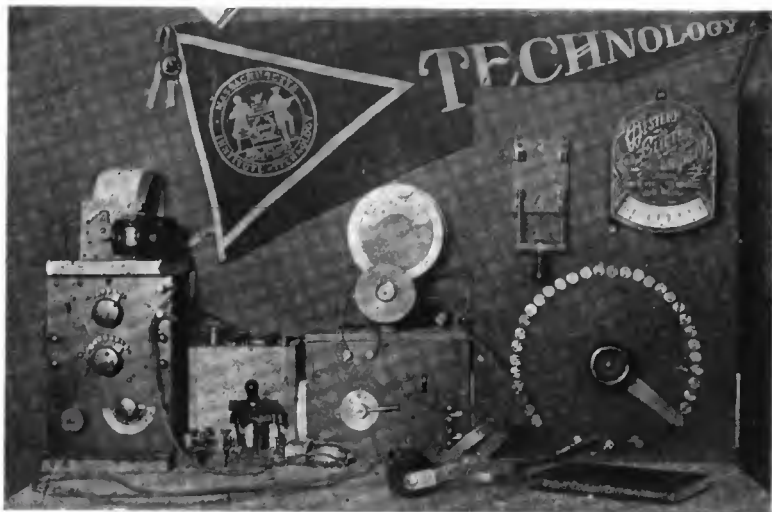
On the extreme right is the control panel which supplies variable D. C. to the plate circuit of the radiophone. In back of the panel is the rectifier (source of supply is 110 v. A. C. lighting current) as well as the filter box, for changing the derived pulsating D. C. to pure D. C. Next in line is the radiophone itself containing the oscillating circuit and power bulb. The microphone transmitter is shown on top. In actual practice, this will be replaced by a regular radiophone microphone. Above the radiophone is the hot-wire ammeter. The rest of the photo needs no description, being the usual receiving apparatus
