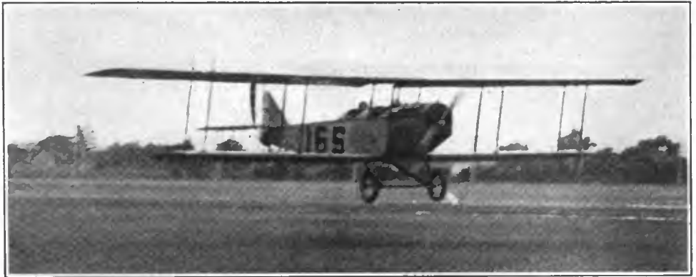
Figure 81—Taxying at the start with wheels on the ground and tail raised
