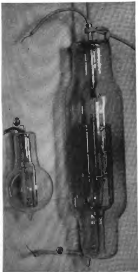
Figure 145—de Forest 0.25 K. W. Oscillation (as compared with type of bulb used in long distance wire telephony)
