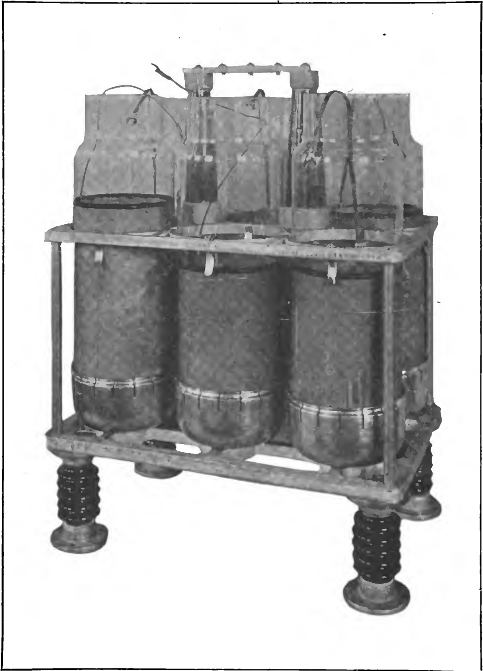
Figure 68.—A battery of copper plated Leyden jars. This unit consists of six jars of .002 microfarad capacity each, making a total value of .012 microfarad, the correct value for a 2 K.W. 500 cycle transmitter. By a special process the inside and outside of the glass are coated with copper, making a very serviceable conducting material which will last for an indefinite period. This is a distinct improvement over the tin foil coated jar which, on account of blistering of the foil, became inoperative after about six months' use. A stranded copper conductor is connected to the inside of the jars and connection is made to the outside through the cups at the bottom. The entire rack is insulated by four electrose insulators
