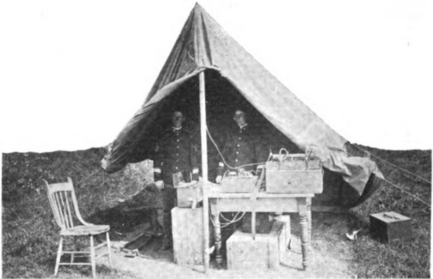
A field equipment of the Signal Corps School set up and working. The apparatus shown here has been superseded by more efficient equipment, increasing the transmitting range and permitting closer wave-length adjustment
