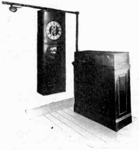
The master clock in the time service department. It operates ninety circuits in New York City on which there are as many as 3,000 synchronized clocks
