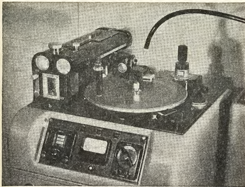
BBC disk-recording machine, of which the turntable, control panel, recording and reproducing head and the traversing-gear housing can be seen. The vertical handle at the back is used to select the turntable speed (78 or 33 \frac{1}{3} revolutions per minute) and the curved pipe is used to suck away the swarf left by the artificial sapphire which is used to cut the groove.
