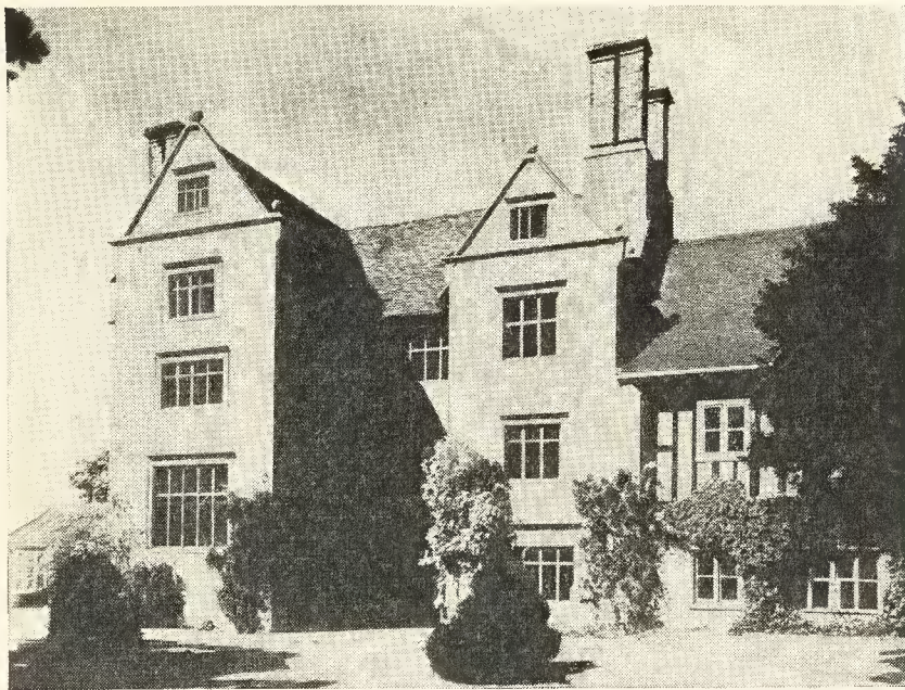
This and the three following illustrations show the results of maladjustments of a television receiver. This picture shows the soot-and-whitewash effect produced by too advanced a setting of the CONTRAST control.
