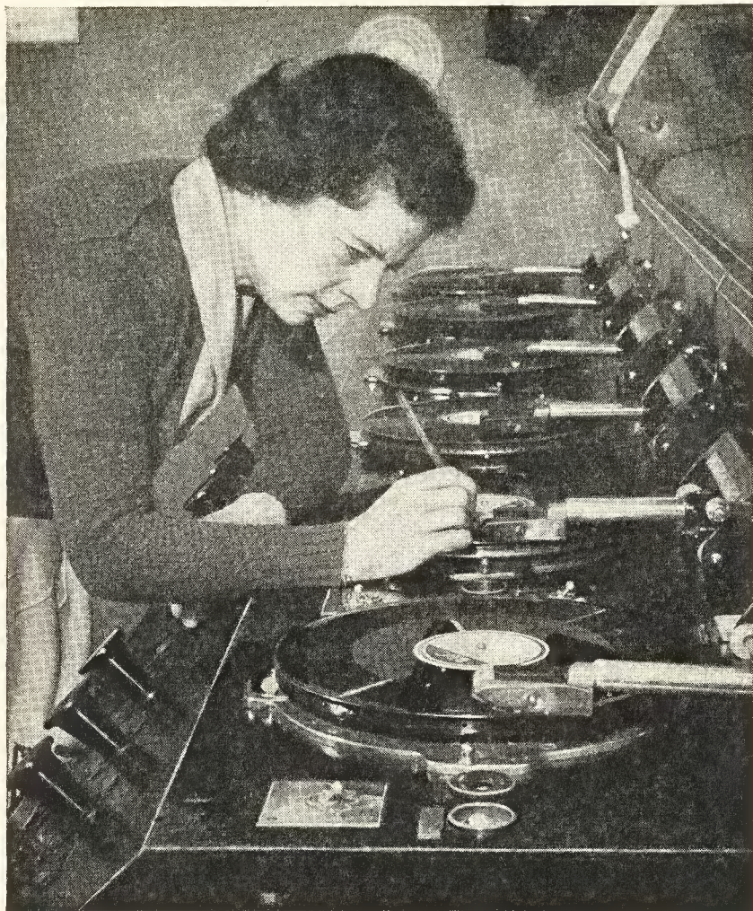
In editing a recording the disk is marked with a yellow wax pencil to indicate the sections of the recording which are to be broadcast. This picture shows one of the many playing desks used by the BBC.
