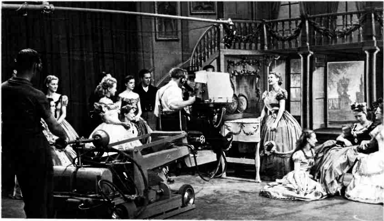
v Motorized camera dolly in action at the BBC's Lime Grove Studios
