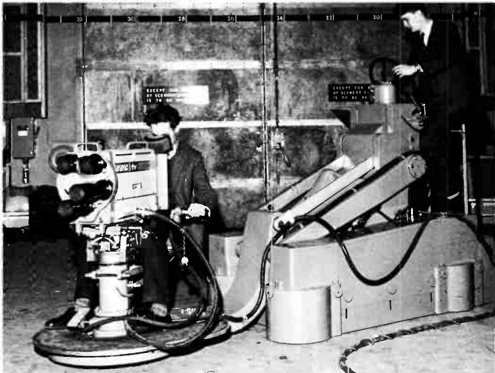
vi Electro-hydraulic dolly, with jib lowered. It can also move sideways ('crab'). Note camera turret and lenses
