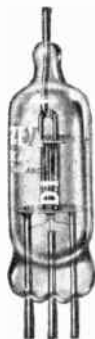
Type D1 Mazda Acorn Diode designed for use in television receivers but adaptable for such purposes as ultra-short wave field strength meters.
