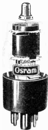
The Osram Z62 is an indirectly heated pentode with a high slope and designed for use in short-wave receivers or wide-band amplifiers. The short seal gives improved performance up to 60 Mc.
