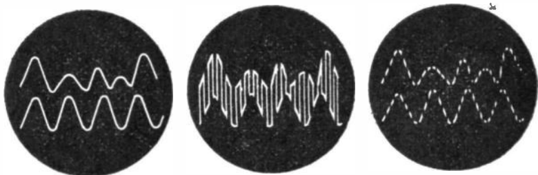
FIG. 22. SHOWING THE DEVELOPMENT OF TWO TRACES WITH THE USE OF AN ELECTRONIC SWITCH
