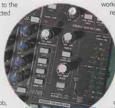
Many switches are of the two-tone 'liquorice allsorts' type, making it easy to see their status
