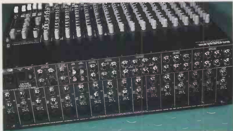
The inclusion of eight direct outs coupled with the four group outputs allows a great deal of flexibility
