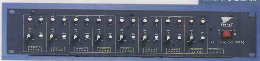
Another interface – this one turns TDIF's into mic channels
