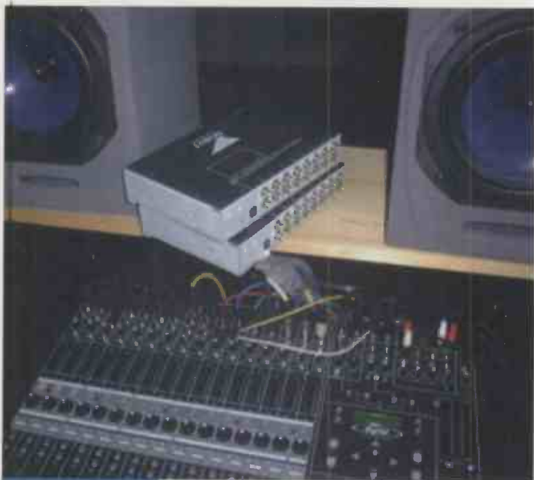
If you haven't got a T/DIF or ADAT connection from your tape machine or computer, you'll need one of Spirit's new interfaces
