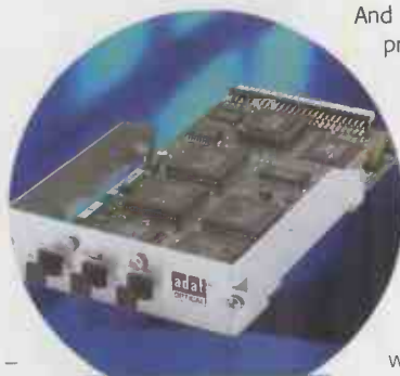
Get the ADAT digital I/O option: 8 ins and 16 outs
