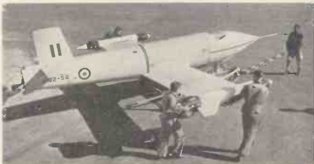
Jindivik—the pilotless target plane—being pushed on runway preparatory to take-off. The wing tip pods contain cameras which record the miss distance of weapons fired against it.
