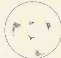
Fig. 6. Pattern on cathode-ray tube screen, showing effect of faulty pre-form
