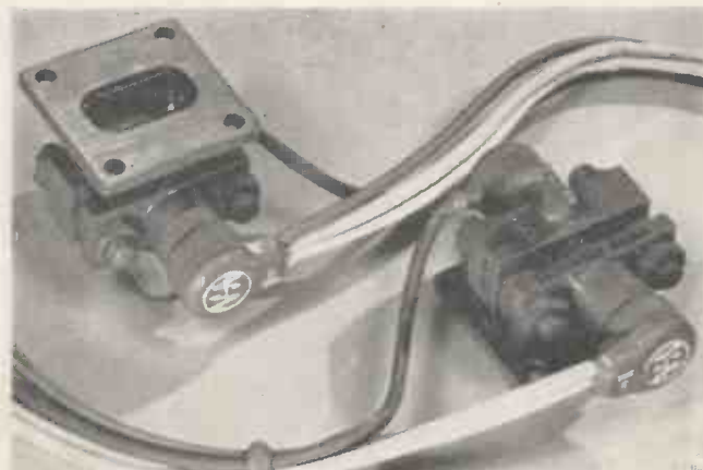
Fig. 15. Klystron tube employing silicone rubber moulding [By courtesy of Varian Associates.]
