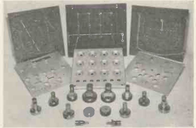
Fig. 2. Templates (top) and some of the tools (bottom) used for producing the three panels (centre)
