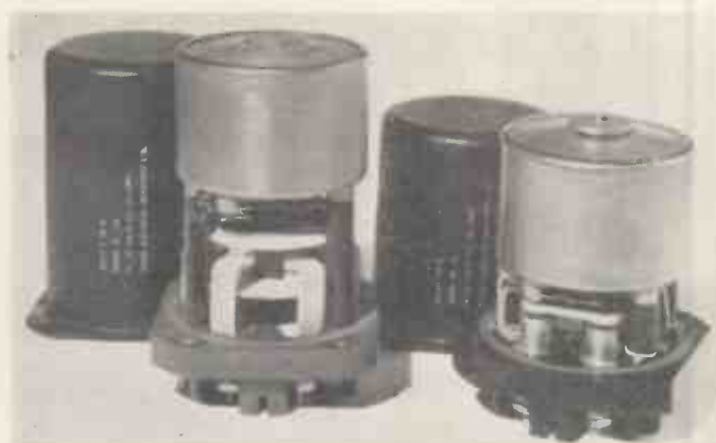
Fig. 12. The coils of these 50A and 100A relays for use in high speed aircraft at ambient temperatures of -75°C to +150°C, are wound with silicone enamelled wire [By courtesy of Thorne Electrical Industries Ltd.]
