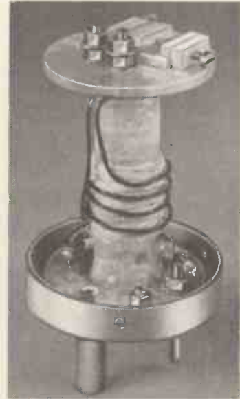
Fig. 5. Measuring transformer with screening can removed
