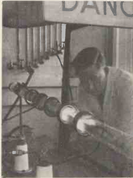
Purification of germanium by zone refining. The germanium ingot is placed in a graphite crucible and the zone is melted by eddy current heating
