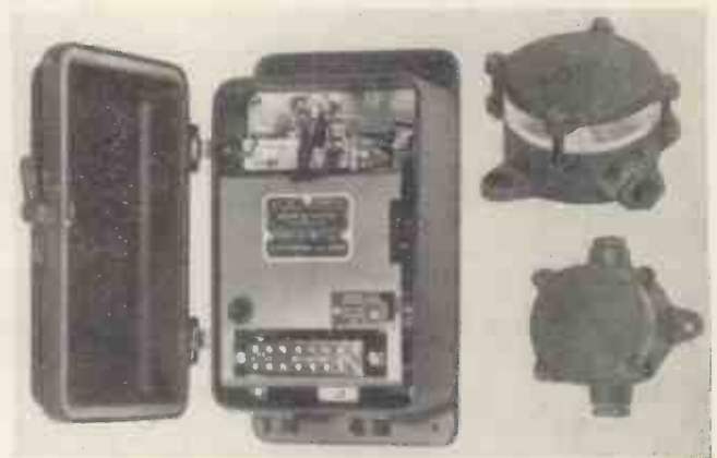
Fig. 6. Automatic lighting controller showing magnetic amplifier and relay in a weatherproof case, and photocell housing
