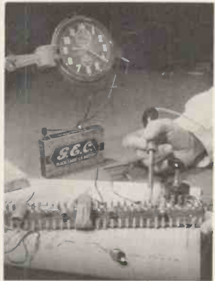
This weather-dependent alarm clock is being developed as an illustration of the uses to which semi-conductor devices can be put. It incorporates a light-sensitive germanium junction photocell with two point-contact transistors as amplifiers. The alarm sounds only if a pre-set brightness level is obtained.
