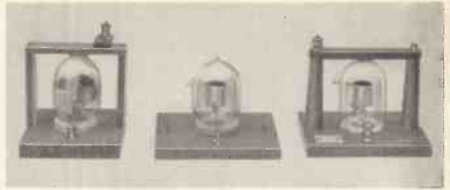
Early Marconi production models of the Fleming diode, forerunner of all thermionic valves.
